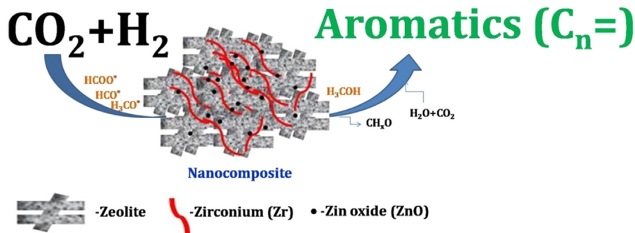
Figure 12.4 Shows the reaction mechanism of CO 2 Hydrogenation over the DFMs catalyst, ZnZrO/ZSM-5. DFMs, dual function materials.
